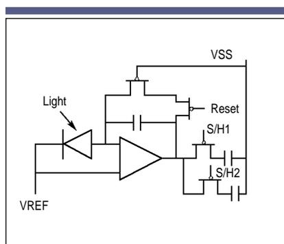
Figure 2. Schematic of an integrating transimpedance amplifier.
