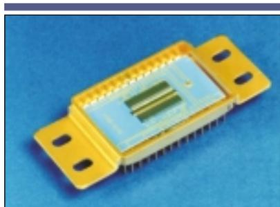
**Figure 3.** An InGaAs photodiode array hybridized to a silicon readout integrated circuit.
