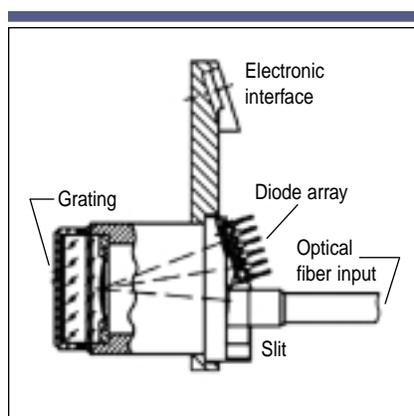
Figure 1. Diagram of a reflection-grating spectrometer with a photodiode array.
