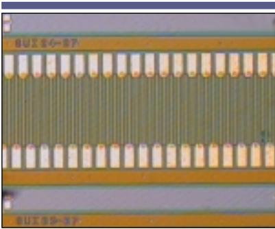
Figure 4. A linear InGaAs photodiode array.
