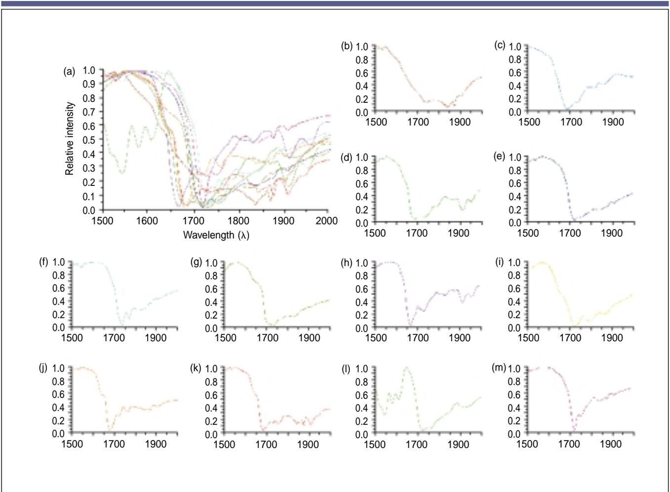
**Figure 2.** NIR absorption spectra of commonly used plastics. Shown are (a) combined absorption spectra and individual spectra of (b) polytetrafluoroethylene, (c) polycarbonate, (d) polymethylmethacrylate, (e) acrylic, (f) polyethylene, (g) polypropylene, (h) polyethylene terephthalate, (i) polyurethane, (j) polystyrene, (k) acrylonitrile-butadiene-styrene, (l) polyamide, and (m) polyvinyl chloride.
