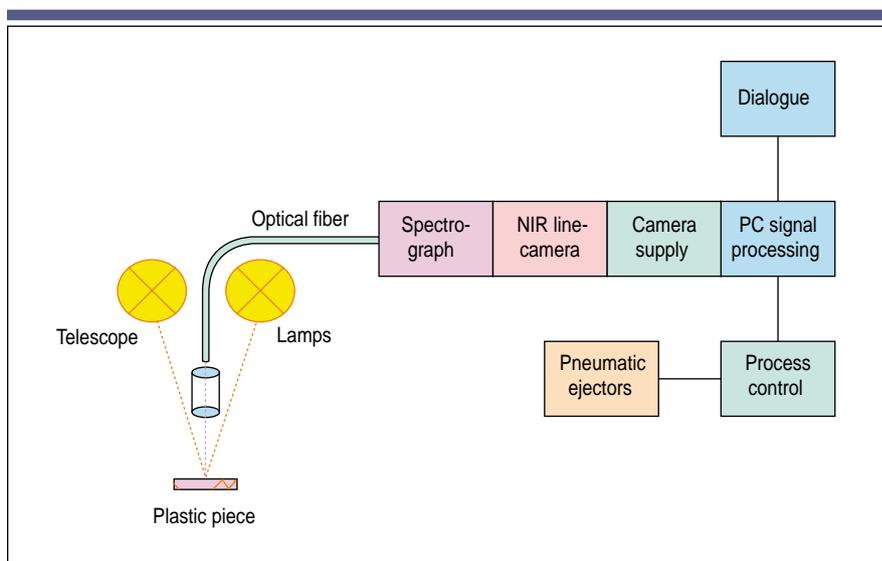
Figure 1. Schematic diagram of an NIR spectrometer.
