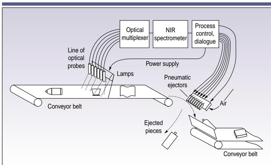
Figure 3. Automated plastic sorting using an optical multiplexer.
