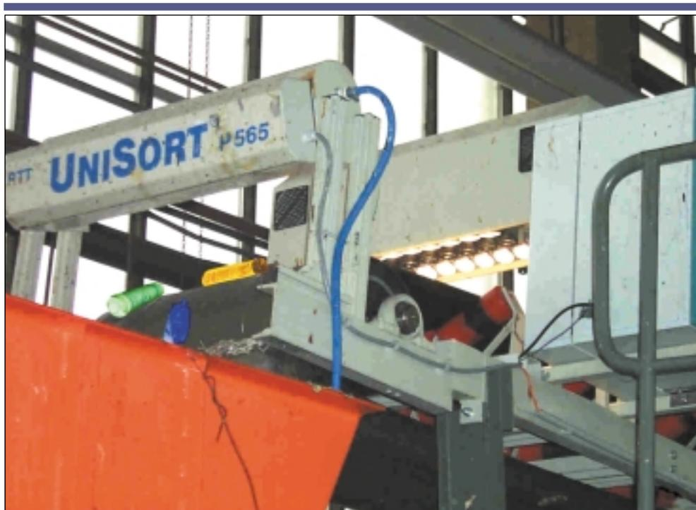
Figure 4. The Unisort system for automated plastic sorting of household waste.
